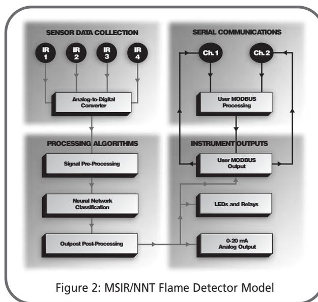
Figure 2: MSIR/NNT Flame Detector Model
